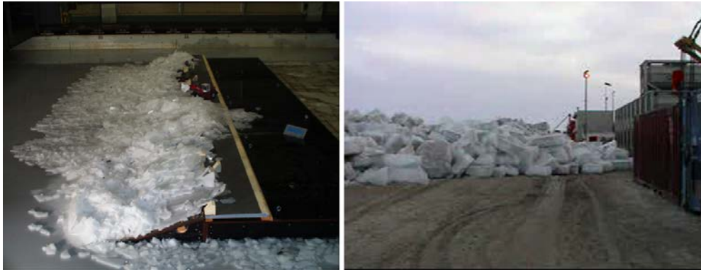
Figure 3: Ice Approaching an Artificial Island (left model test – right full scale)
