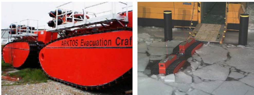
Figure 4: Arktos amphibious vehicles evacuation crafts (left: full scale – right: model tests)
