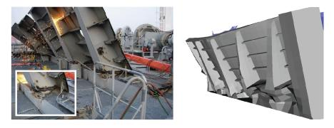
Figure 16: Comparison of actual collapsed breakwater (left) with numerically predicted one (right) (Heo *et al.*, 2010)
