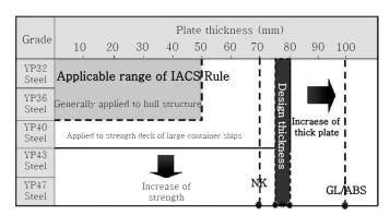
Figure 3: Recent history of thicker and stronger steel plates for large container ships – An *et al.* (2010)
