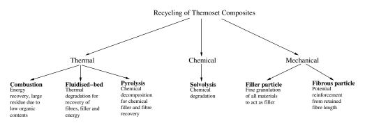
Figure 5: Recycling methods for thermoset composites – Pickering (2006)
