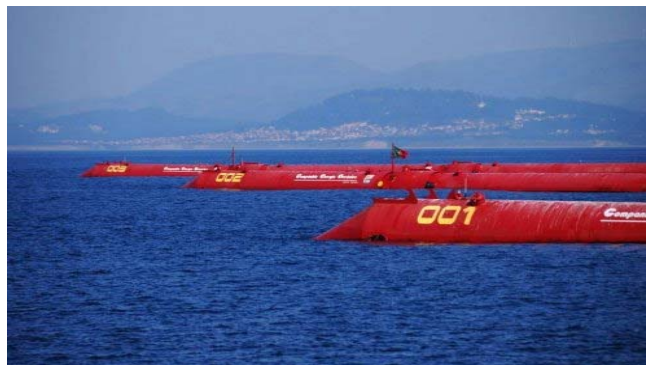
Figure 6: Three P1-A Pelamis machines with capacity of 2.25MW, 5 km off the west coast of Portugal (substation of Aguçadoura).
