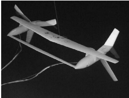
Figure 14: Aquantis 1/30th scale C-Plane prototype in position for a tow test.
