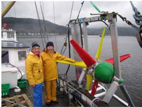
Figure 21: Demonstrator (CoRMat) on launch vehicle St. Hilda, Clarke, et al. (2007).
