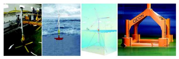
Figure 6. Concepts of TLP or TLB floating wind turbines (from left: a) Iberdrola TLP (Rodriguez et al., 2014); b) Glosten PelaStar TLP (Scott, 2013); c) TLB concept (Myhr and Nygaard, 2012); d) GICON-TLP (Adam et al., 2014)).
