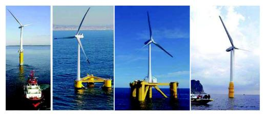
Figure 5. Prototypes of floating wind turbines (from left: a) Hywind (Statoil, 2014); b) WindFloat (PrinciplePower, 2014); c) Fukushima semi-submersible (FOWC, 2013); d) GOTO spar (GOTO-FOWT-Website, 2014)).
