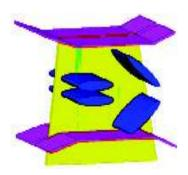
Figure 9. A dual foil arrangement in the WIGT concept (Liu, 2012b).
