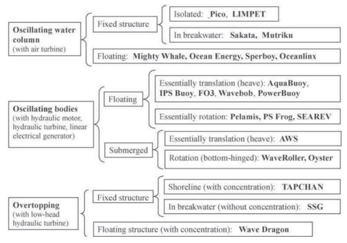
Figure 8. Wave energy technology classification (Falcão, 2010).
