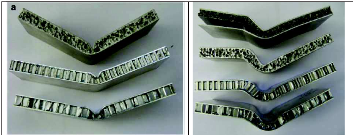
Figure 6. Collapse modes of investigated honeycomb and aluminium foam sandwiches obtained by static bending tests (Crupi et al., 2013)
