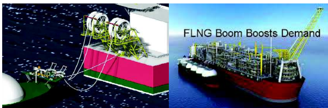
Figure 11. Possible LNG-FLNG tandem configuration using Dynamic Positioning next to traditional side-by-side solution (Prelude) (see www.eshiptrading.com )
