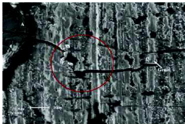
Figure 1. Fatigue crack path resulting from the coalescence of three individual discontinuities: a notch (A), a corrosion pit (B) and a grain boundary (C).
